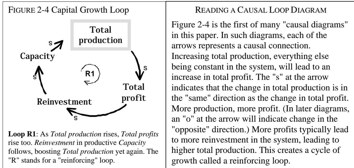
equipment —sawmills, tractors, fishing boats — which is then used to increase total production. In this growth process production leads to more capacity for production.
